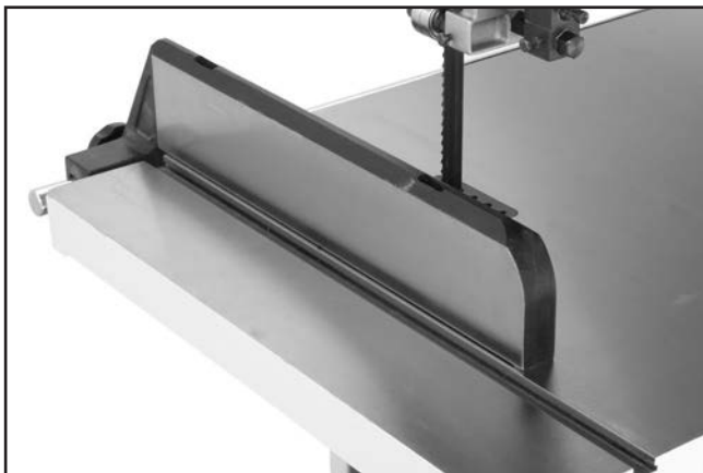
Figure 56. Example of fence parallel with miter slot.
