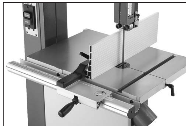
Figure 23. Example photo of correctly installed fence.
