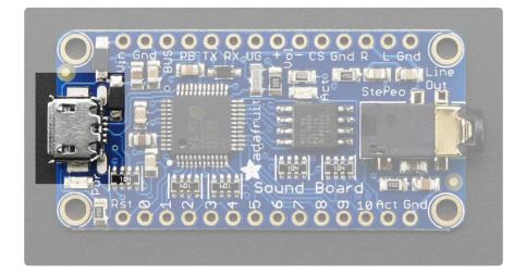
Starting from the left is the micro USB jack. You'll need a standard MicroUSB cable to connect this to your computer. You do need a computer (any will do) in order to save files onto the Sound Board flash storage
