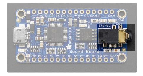
All the way to the right is the headphone jack. This is for connecting to a pair of headphones or into a powered speaker. It cannot drive an 8 ohm or 4 ohm speaker. Instead, an amplifier will have to be used (basically, just like your phone or pocket MP3 player needs an external powered/amplified speaker)
