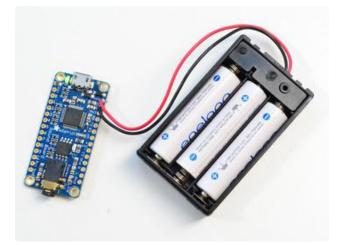
The nicer battery packs have switches, or you can just remove the batteries when not in use. If the green light is lit, it's powered up!
