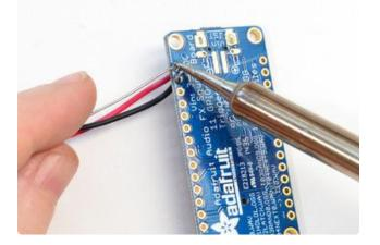
Solder both wires securely. You cannot just twist the wires into place!
