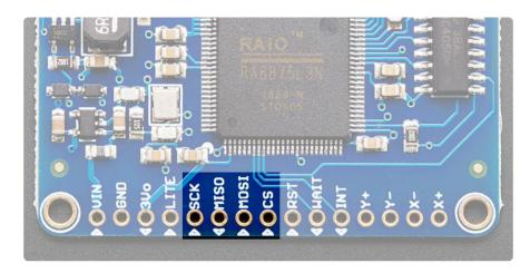
All pins are 3-5 V compliant, so you can use with 3V or 5V micocontrollers
