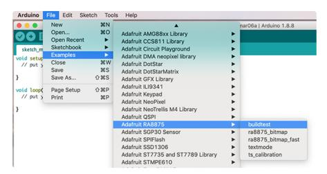
Be sure to set the screen size in the sketch to the appropriate size and upload it to your Arduino
