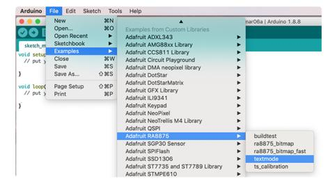
Just like the previous example, be sure to set the screen size in the sketch to the appropriate size and upload it to your Arduino
