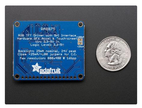
The RA8875 can also handle standard 4-wire resistive touchscreens over the same SPI interface to save you pins. There's an IRQ pin that you can use to help manage touch interrupts. The touchscreen handler isn't the most precise driver we've used, so we broke out the X/Y pins so you can connect them up to something like the STMPE610 which is a very classy touchscreen controller. (http://adafru.it/1571)
